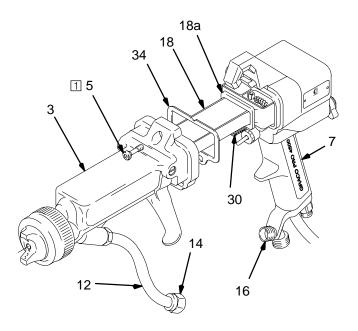
Tighten to 18 in-lbs (2 N•m) **maximum** (about half turn past snug), using wrench provided.
